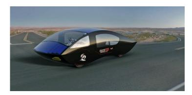
SunSPEC4 is Singapore Polytechnic's fourth solar car, and its first two-seater model. Designed and built completely in-house, SunSPEC4 resembles a futuristic saloon car – albeit one powered solely by solar cells. In contrast to the polytechnic's previous solar models, SunSPEC4 is designed to perform similarly to a standard commercial car in terms of speed, seating capacity, and range.
